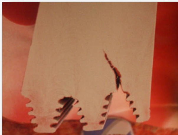
Figure 4: Macro view of the crack after penetrant test.
