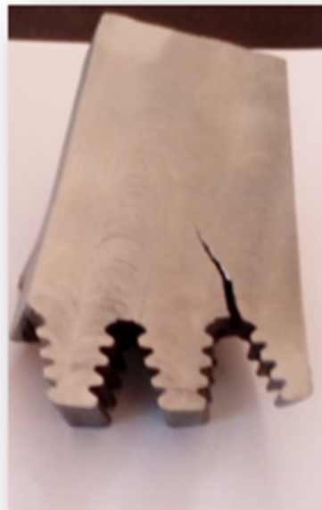
Figure 2: Macro view of a crack formed in a gas turbine blade.
