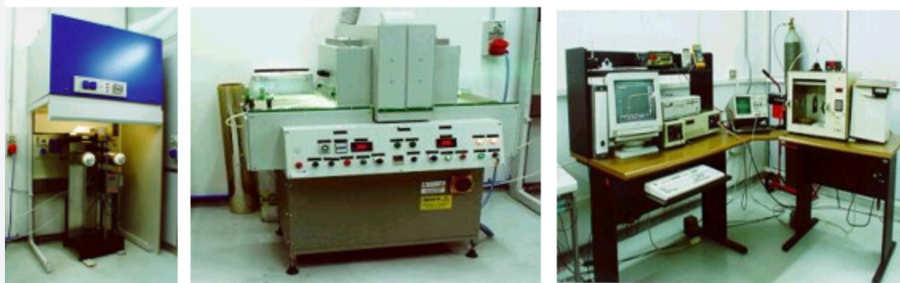
Figure 1: PDLC coater/laminator (left), UV curing conveyor (middle) and electro-optical system (right).
