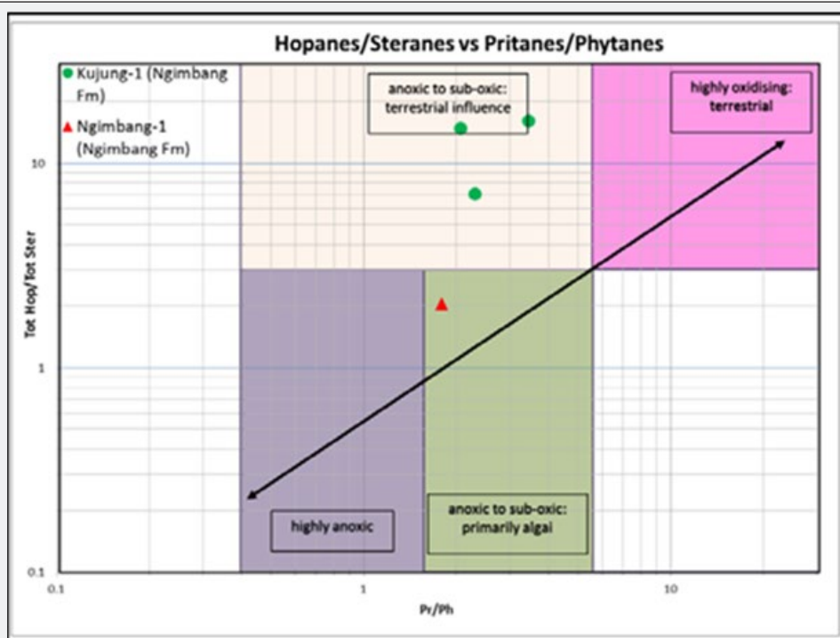
Figure 5: Plot of hopane/sterane versus pristane/phytane showing the organic source input and the environment condition of rock samples.
