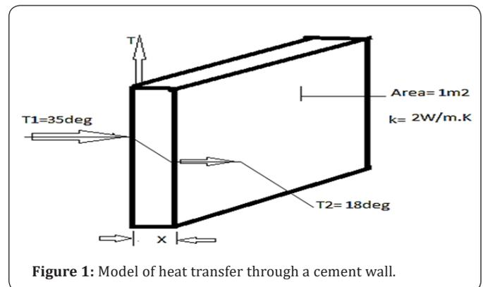
Figure 1: Model of heat transfer through a cement wall.
