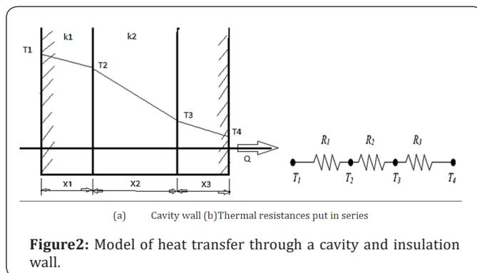
Figure 2: Model of heat transfer through a cavity and insulation wall.
