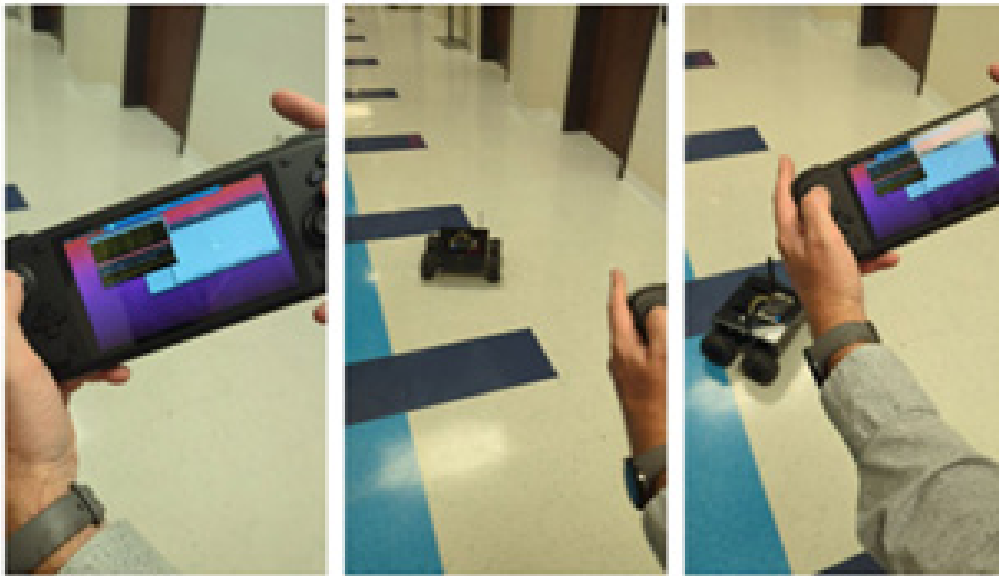
Figure 10: AYN Loki as a ROS Based Teleoperation Device.
