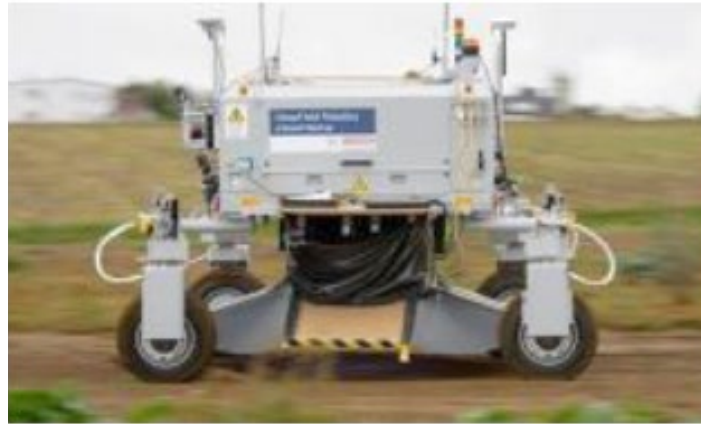
Figure 6: Weeding robot designed by BoniRob in German.
