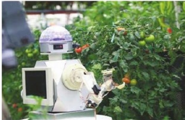
Figure 3: Tomato picking robot designed by Panasonic Company in Japan.
