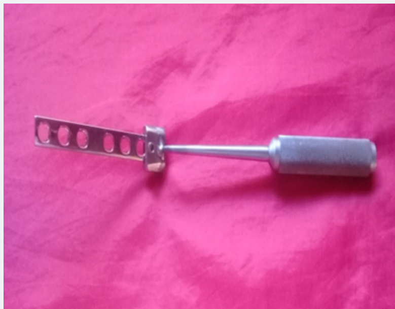
Figure 2: Own sheet holder, designed by our service team.
