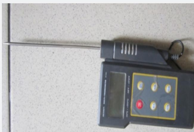
**Figure 2:** Multi thermometer DT300.
