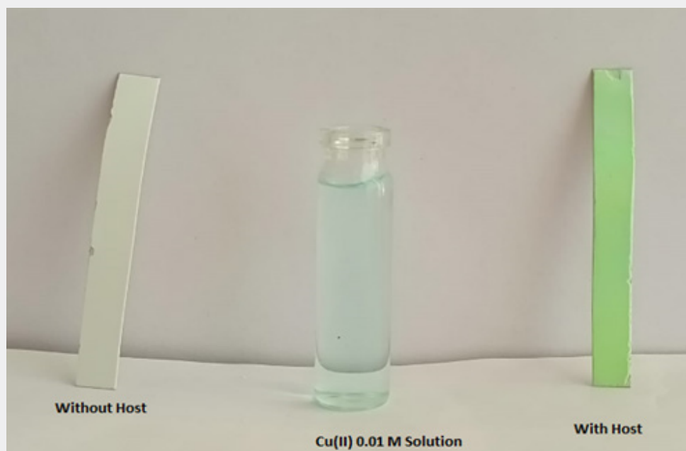
Figure 7: Practical application of 6-TP in presence of Cu(II) by test strip (silica TLC plate).
