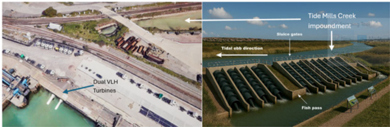
Figure 1: Conceptual reinstatement of Tide Mills Creek incorporating dual VLH turbines (based on image prepared by Phil Nutley, [University of Brighton/ Nevermind Global Limited], reproduced with permission) and Archimedes screw turbines, together with sluice control and fish-pass provision.
