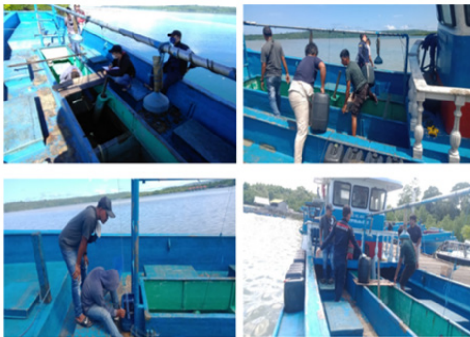
Figure 9: Inclining test of Skipjack Pole and Line MV. Yora 01.
