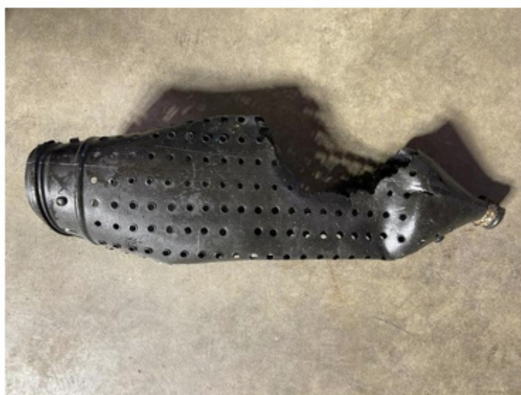
Figure 8: Eel trap tube with a piece missing thought to be due to a bite by a shark. Photo courtesy Dr. Sarah-Jeanne Royer.
