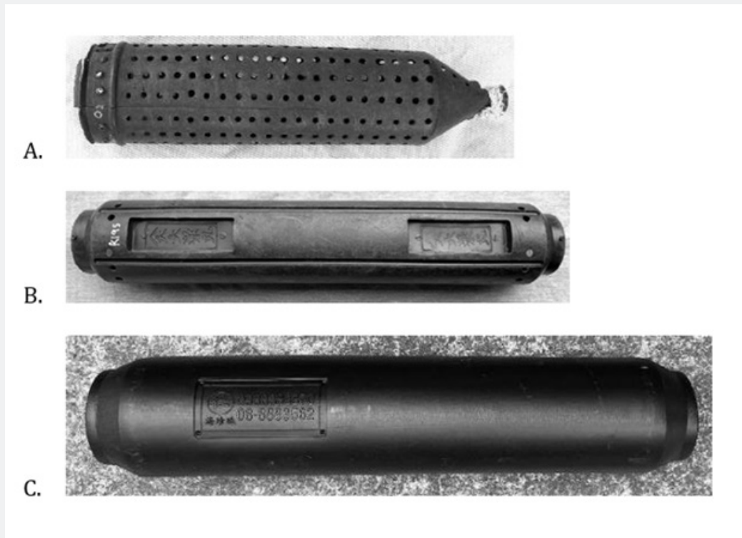
Figure 3: Examples of eel trap tubes (ETT) used in the western North Pacific Ocean (NPO). Eel trap entrances (ETE) are attached at one (A) or both ends (B, C). Average length: A) 51-55 cm, B) 70-75 cm, C) 107 cm.
