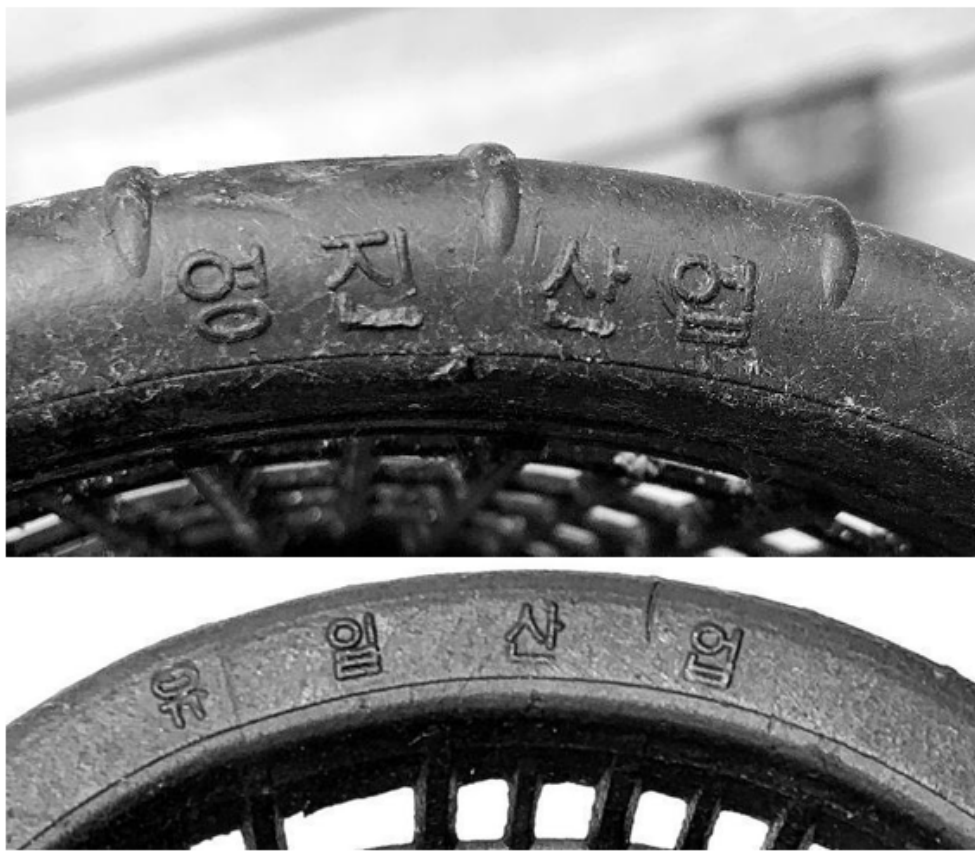
Figure 13: Examples of markings on rims of eel trap entrances (ETE) identifying the manufacturers. top: 영진산업 Youngjin Industry. bottom: 유일산업 Yooil Industry.
