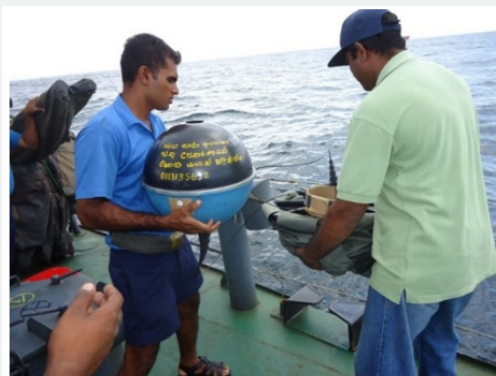
Figure 2: Deployment of SVP drifters in the south of Sri Lanka.
