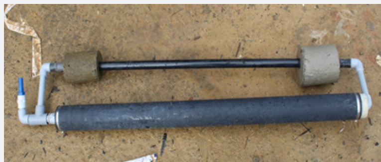
Figure 1: Airstone with concrete sinks having 0.3 mm air hole, 1.5 m length and 3-inch diameter.
