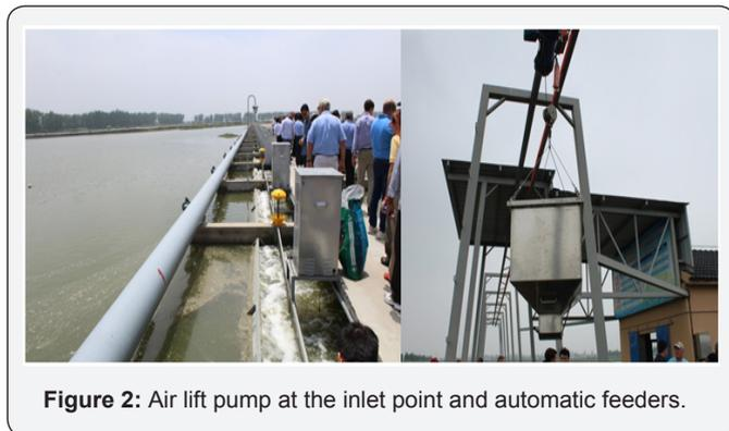
Figure 2: Air lift pump at the inlet point and automatic feeders.
