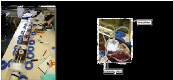
Figure 4: The in vitro set up. With five different situations; one control, two meat pieces inoculated with S. aureus in a dry environment DC & AC, two meat pieces inoculated with S. aureus in a wet environment.
