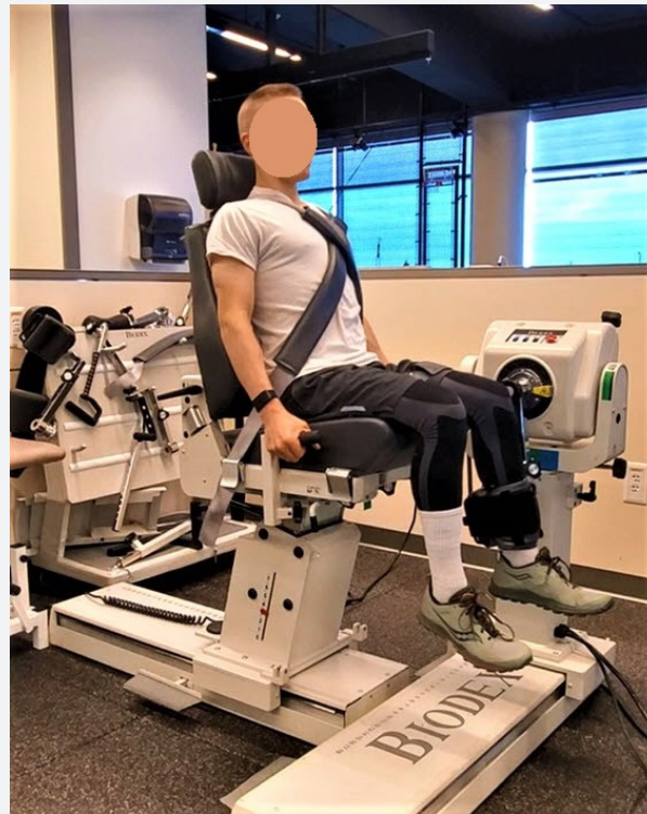
Figure 1: Knee extension isometric testing set up on Biodex System 4 Pro
