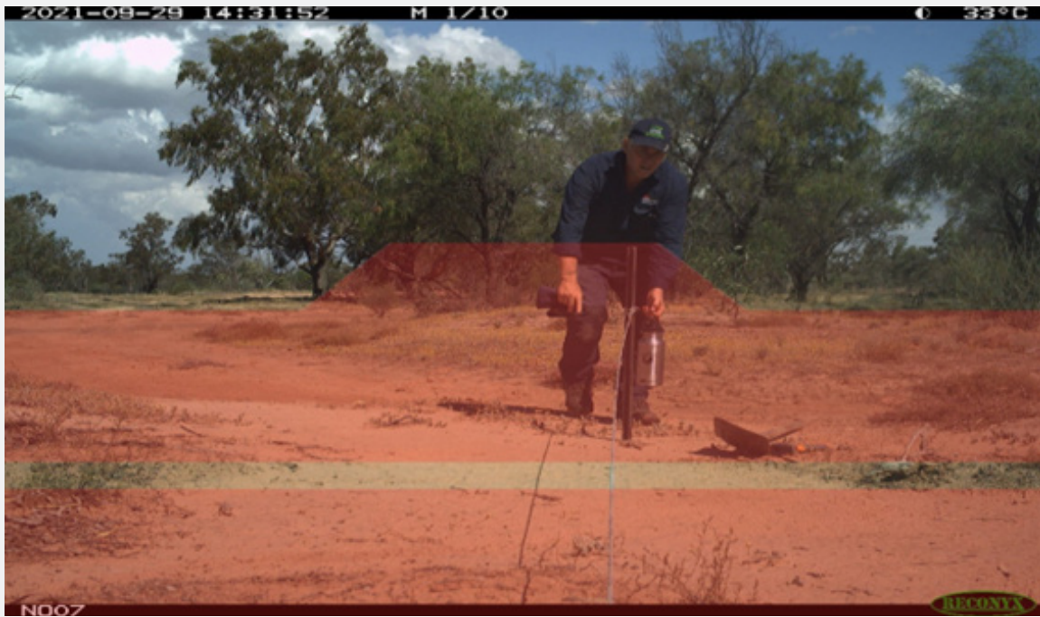
Figure 5: During hot conditions when the background-human temperature differential is not significant to trigger the PIR, a cooler temperature item like a cold-water bottle from the car fridge will also trigger the PIR.
