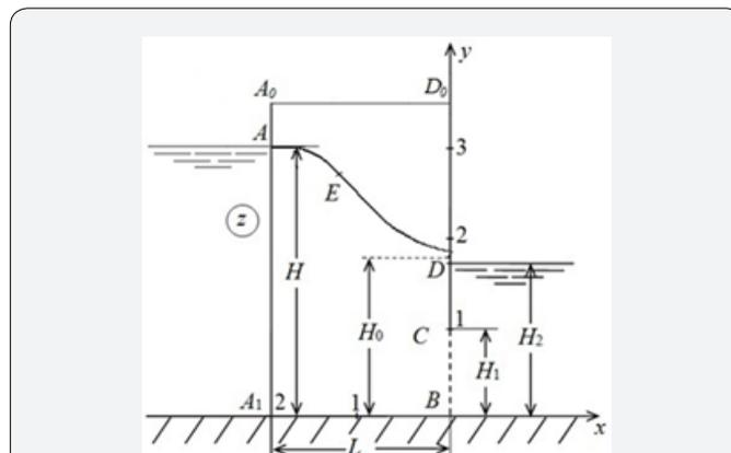
Figure 2: The Current Picture in a Rectangular Jumper Calculated at  $\epsilon = 0.5$ ,  $H = 3$ ,  $L = 2$ ,  $H_1 = 1$ ,  $H_2 = 1.4$ .
