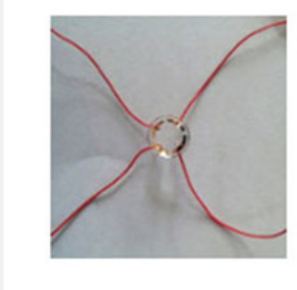
Figure 5: Lens used in the study in Grimnes configuration [9] for posterior chamber analysis and in Focus impedance Measurement [15] for anterior chamber analysis.
