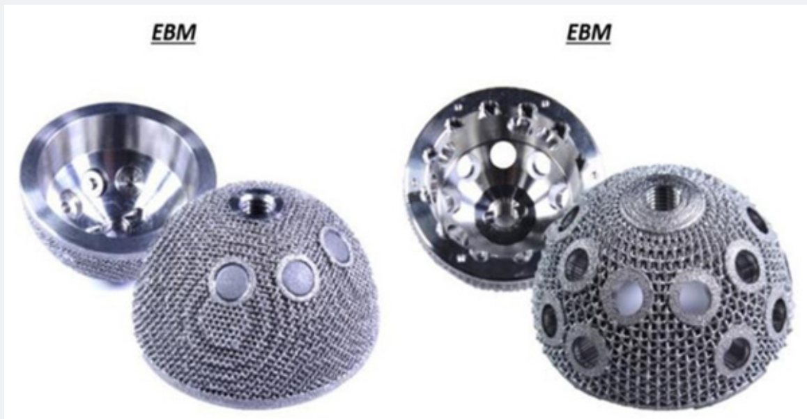
Figure 4: Porous titanium alloy acetabulum cup prepared by EBM [13].
