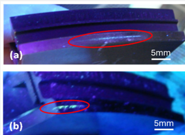
Figure 2: FPI Inspection of MCrAlY Coating applied on a Ni-based alloy part. (a) Linear defect associated with potential coating delamination at the interface is indicated in the middle section of the coating; (b) Similar linear defect is observed at a corner of the coating specimen.
