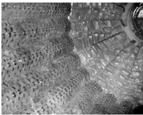
Figure 5: Rubber lining with sealed air cavity for operation with balls with a diameter of 100mm.
