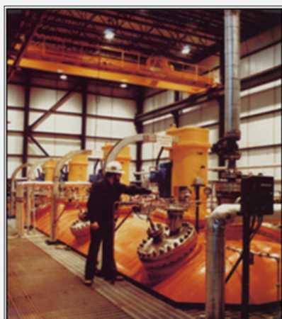
Figure 8 : Pressure leaching process for zinc sulfides.
