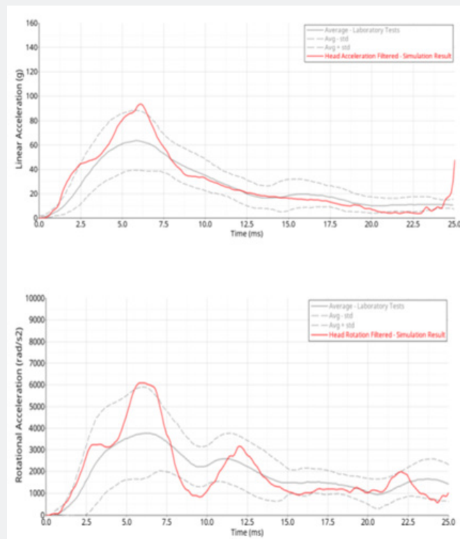
Figure 15: Case 3-Striking player Hybrid III model response vs tests.
