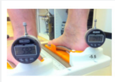
Figure 6: The print will show in what position and at what height of the heel the arches of the feet are in a neutral position and what is the difference in leg lengths (Huk).
