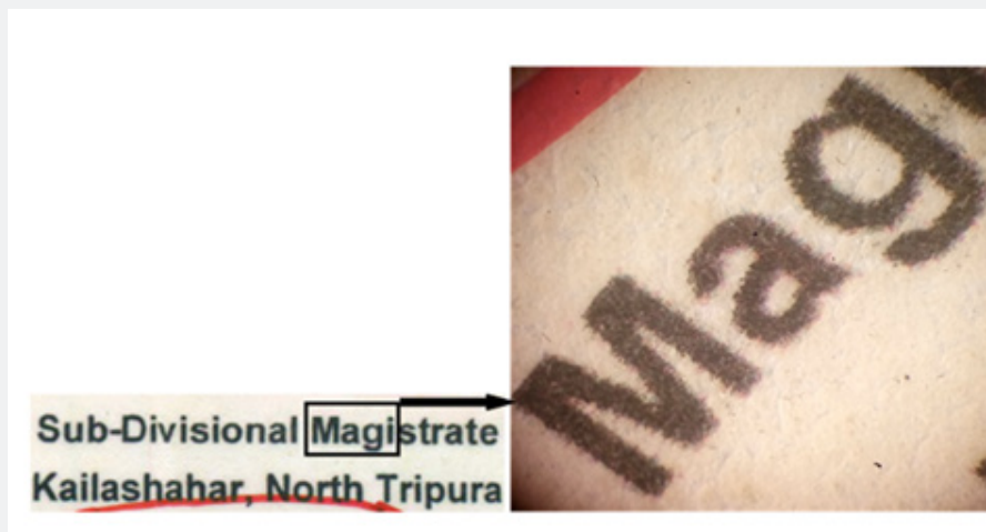
Figure 3: Suspected PRTC shows satellite colour dots that appear on both sides of the characters are indications of inkjet printing.
