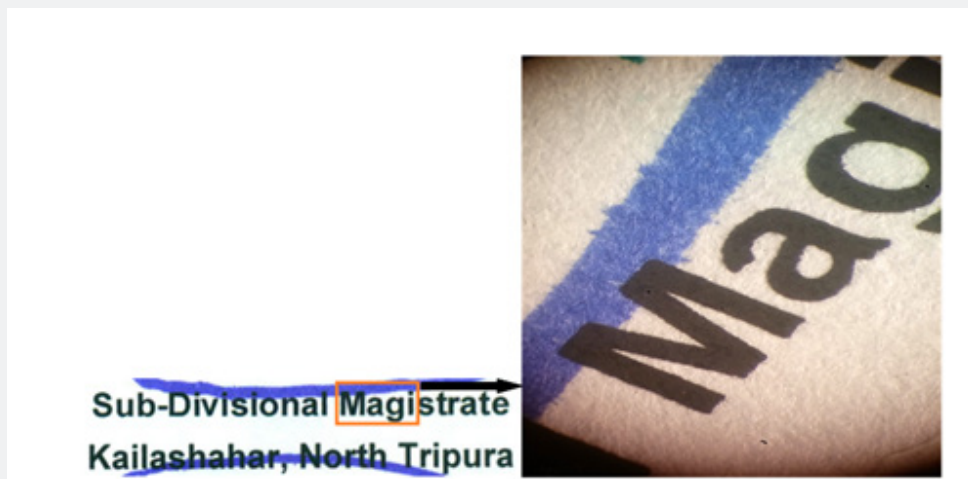
Figure 4: Original sample of PRTC shows sharp and fine edges of letters indicate that the document is printed by laser printing process.
