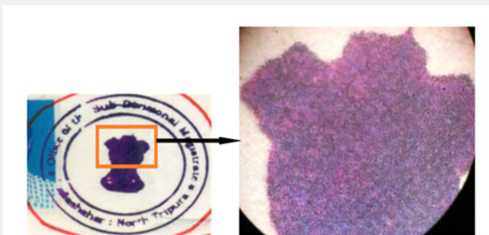
Figure 5: Manipulated rubber stamp impression of the sub-divisional magistrate under higher magnification of suspected PRTC.
