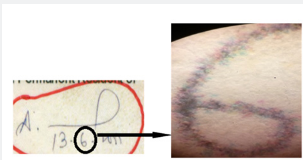
Figure 2: Under magnification of the suspected PRTC the above image (Signature of issuing authority) shows the absence of ink, striation marks or grooves, presence of droplets of ink. This indicates that the signature is a scanned signature and produced by an inkjet printer. This image also shows a typical four colour (cyan, magenta, yellow and black) dithering pattern associated with an inkjet-printed colour graphic.
