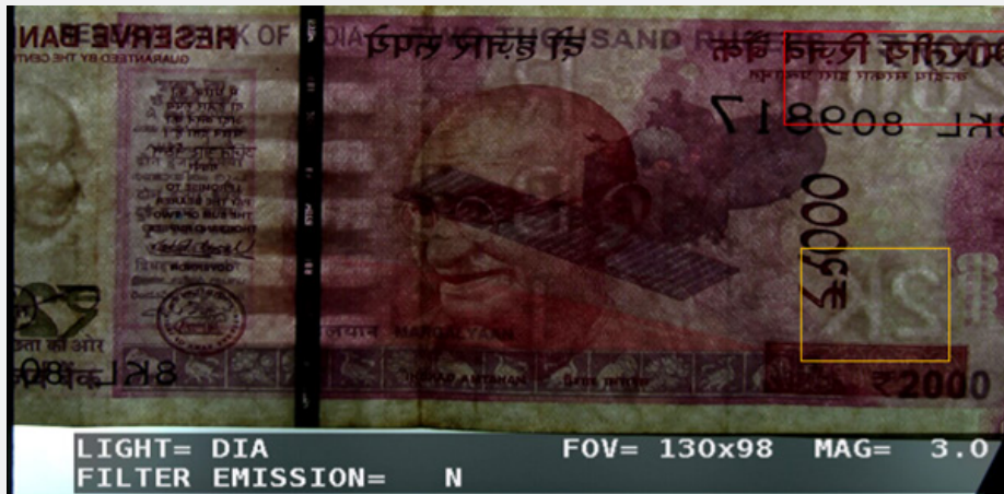
Figure 5: Paper currency note of Rs. 2000 showing RBI secret watermark 2K and 2000 under DIA light source.
