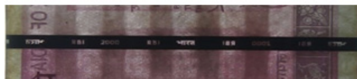
Figure 11: Paper currency note of Rs. 2000 visualised under DIA filter which displays security thread in black colour along with the micro letters.
