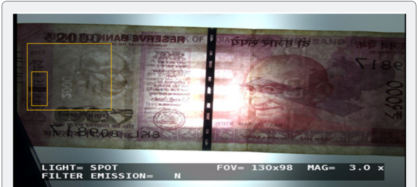
Figure 2: Paper Currency note of Rs. 2000 showing watermark (1) of the Mahatma Gandhi Portrait and electrotype watermark (2) under SPOT.
