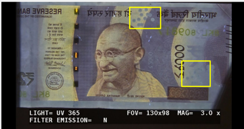
Figure 23: Paper currency note of Rs.2000 displaying Omron features present on obverse side under 365 nm UV light.
