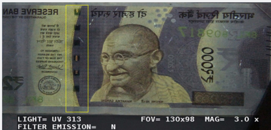
Figure 6: Paper currency note Rs.2000 showing fluorescent feature by security thread on the obverse side in 313nm UV light.
