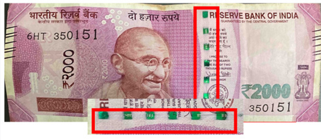
Figure 4: Paper currency note Rs. 2000 showing green colour security thread in visible light.
