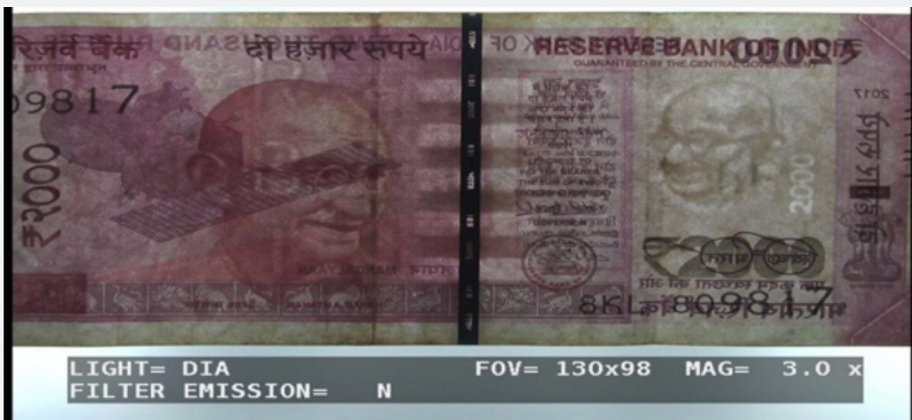
Figure 10: Paper currency note of Rs.2000 showing micro letters RBI and 2000 and BHARAT in Hindi on security thread which is fully embedded and continuously readable on the reverse side.
