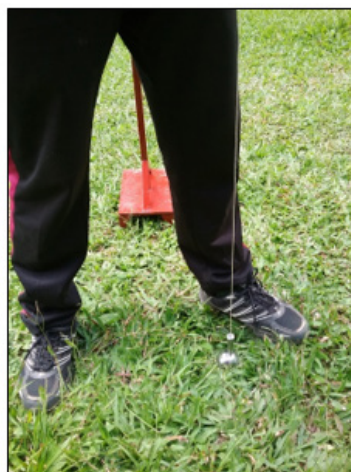
Figure 4: Plumb bob hooked to trigger guard of the rifle was used to align the ejection port of the rifle to the 0 point of the grid system.
