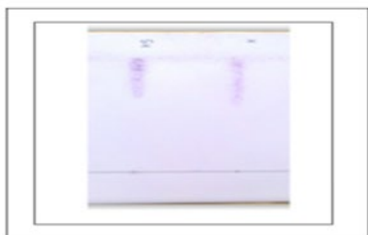
Figure 6: TLC for Standard Kerosene and Completely Burned Cloth.
