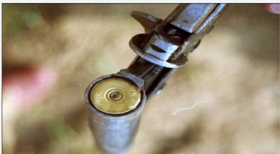
Figure 5 : The fired cartridge (KF 12) case inside the barrel of country made pistol.
