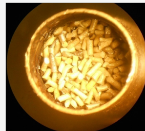
Figure 6: Microscopic view of dry propellant inside the standard cartridge case.
