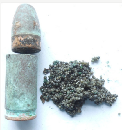
Figure 3: Moist Propellant of a 9 mm dumped ammunition.
