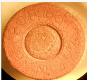
Figure 2: Head stamp of one representative 9 mm dumped ammunition.
