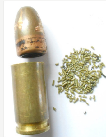
Figure 4: Propellant of a 9 mm standard ammunition.
