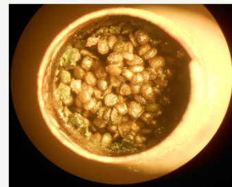
Figure 5: Microscopic view of clustered propellant inside the dumped cartridge case.
