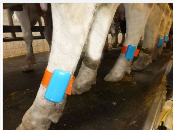
Figure 3: Accelerometers can readily detect changes in locomotion significantly earlier than simple human observation
