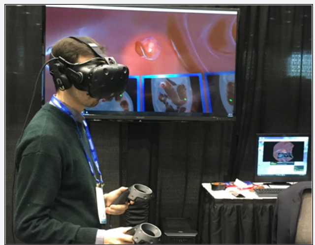
Figure 3 : Trainee navigates reconstructed CT scan demo in medical virtual reality (MVR) environment using an immersive head-mounted display (HMD) on HTC Vive™ headset. The field of vision combined with handheld controllers enables exploration and manipulation of the model, which is viewable in 2D to bystanders on the adjacent monitor. MVR systems can be used to explore model patients or specific physiological environments generated from unique imaging data like MRI and CT scans.
