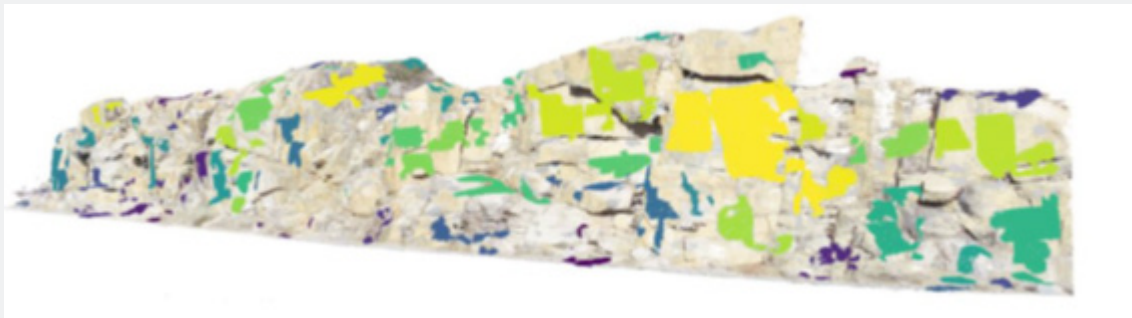
Figure 4b: DBSCAN is used for identifying joint planes by clustering the segmented point cloud [2].
