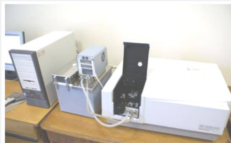
Figure 3: An Instrument setup of RF-5301 PC Spectrofluorophotometer.
