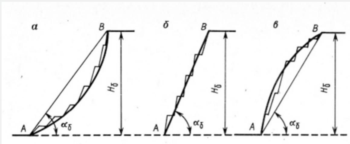
a - concave; б - flat; в - convex;  $\alpha_б$  - the angle of the side of the quarry;  $H_б$  - side height
