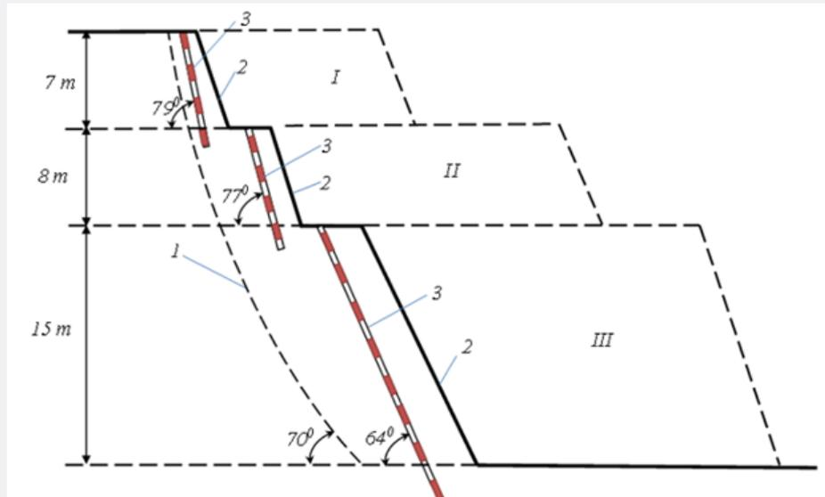
1 - the final contour of the quarry; 2 - the slope of the ledge of the quarry; 3 – the inclined contour well; I - the upper horizon; II - the middle horizon; III - the lower horizon
