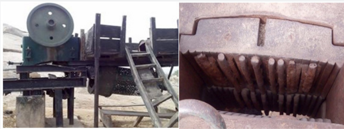
Figure 2: Moribund jaw crusher in Jalingo quarry [4].
