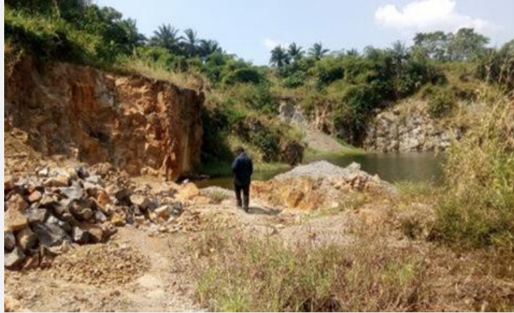
Figure 5a: Field Photograph of the mining pit with 3m to 5m overburden materials removed, of different types of dolerites, dark, spotted, grey and weathered at Obiulo-Lekwesi mine.
