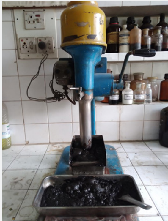
Figure 1: Laboratory Flotation Machine (Model: D-12, Make: Denver, USA).
