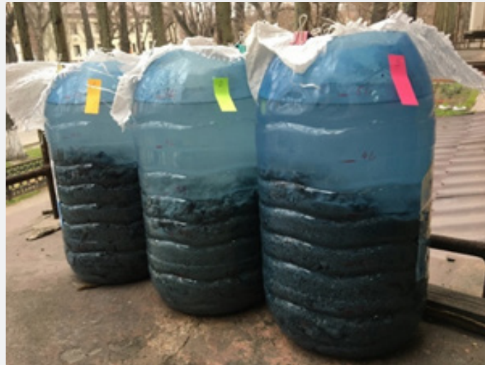
Figure 3: Containers with ferrous slags mixed with control water for studying physical and chemical properties of contact water.
