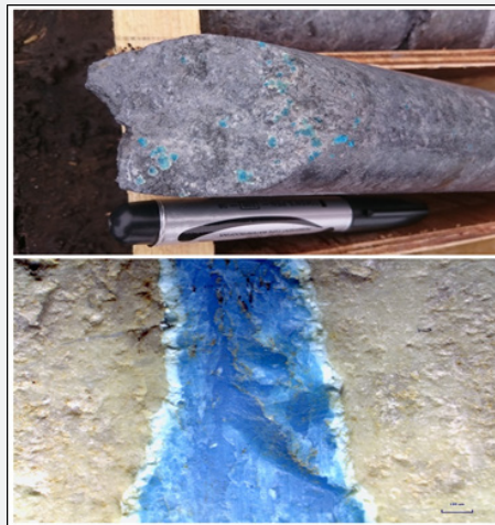
Figure 7: Turquoise ( \text{CuAl}_6(\text{PO}_4)_4(\text{OH})_8 \cdot 4\text{H}_2\text{O} ) Mineralization in the Reza Gold Deposit: Turquoise Minerals observed on Fractures, Rhyodacite core piece (the upper); Turquoise Mineral Fragment in Rhyodacite rock, photos taken under Leica S8AP0 Binoculars (the following).
