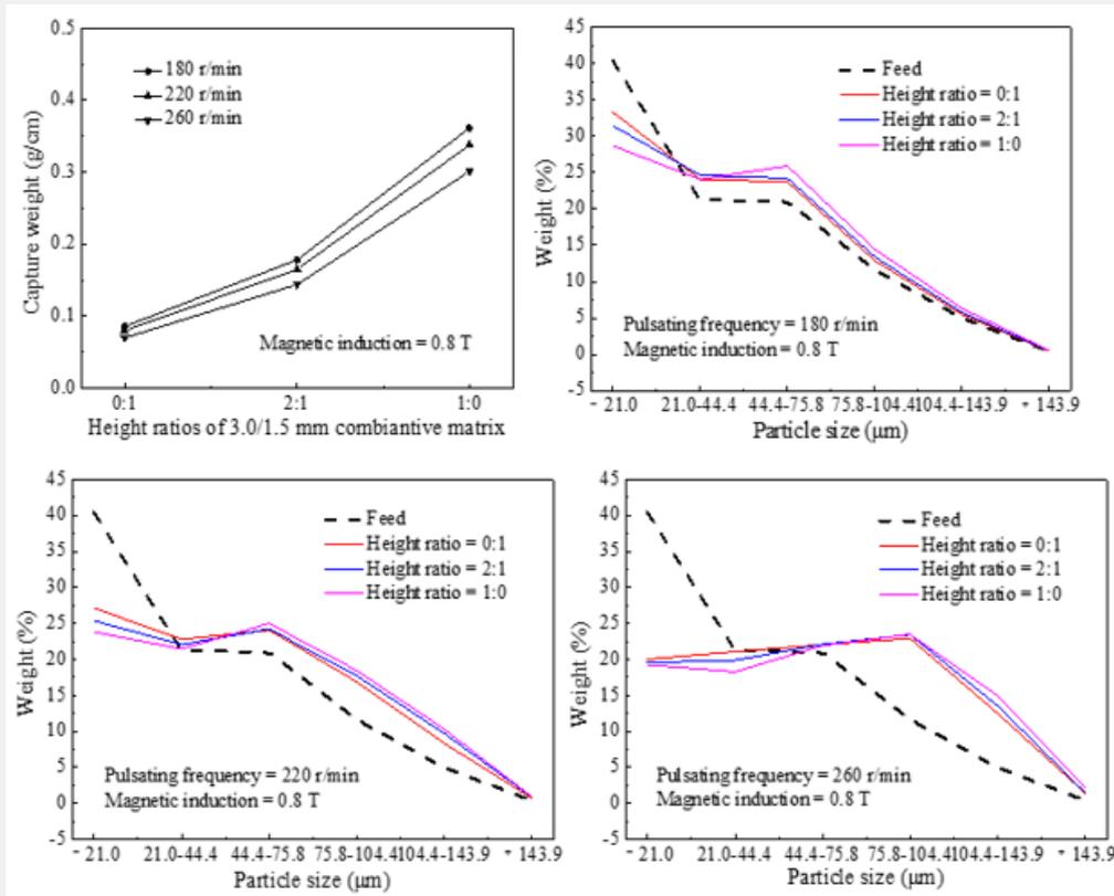
Figure 5: Effect of Pulsating Frequency on Capture performance of 3.0/1.5mm Combinative Matrix.
