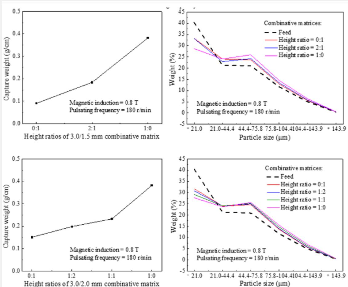
Figure 3: Capture performances of 3.0/1.5mm (up) and 3.0/2.0mm (down) Combinative Matrices.
