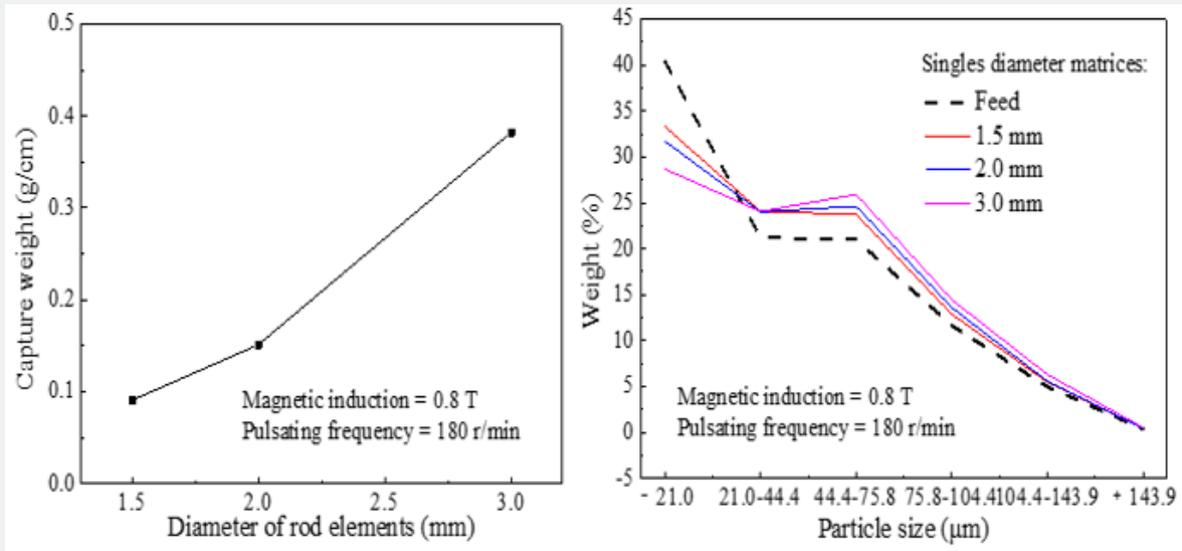
Figure 2: Capture performance of 1.5mm, 2.0mm and 3.0mm single Diameter Matrices.
