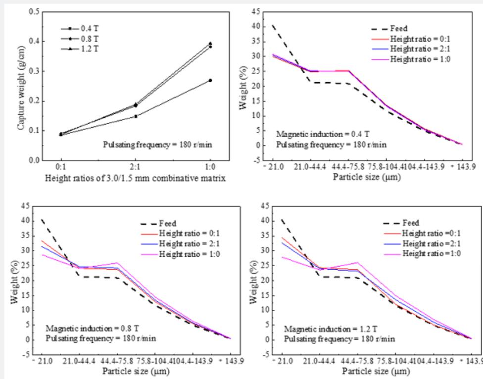
Figure 4: Effect of Magnetic Induction on Capture performance of 3.0/1.5mm Combinative Matrix
