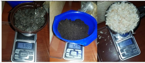
Figure 4: Weighing of samples of RDF-raw materials (a), peat (b), and sawdust (c) to create formulations in containers.
