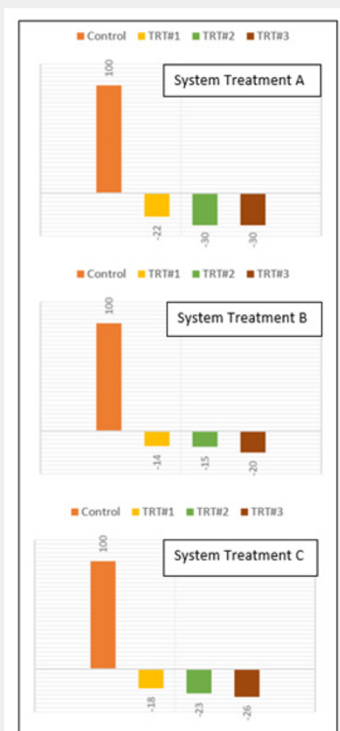
Figure 2: Graph of hydrocarbon destruction efficiency in Systems Treatment A, B, and C for soil Sample 2.
