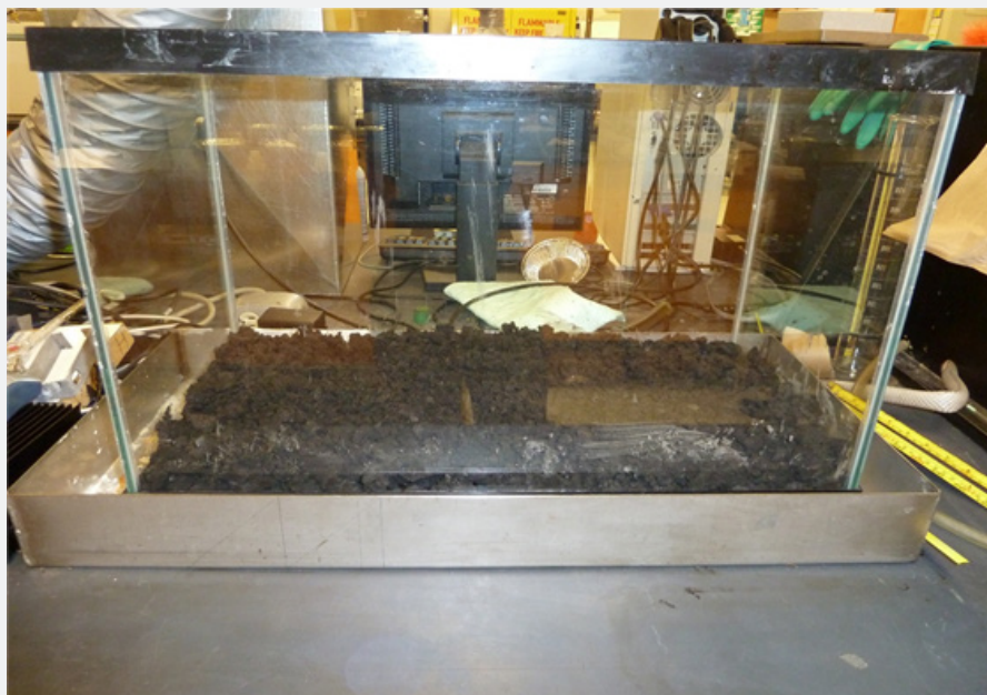
Figure 1: Experimental setup for pyrite oxidation tests in a glass tank.
