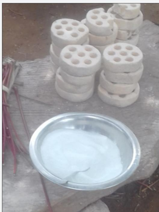
**Figure 4:** Broken bottles ground into powder to be baked into beads [5].
