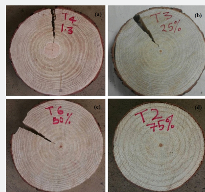
Figure 1: Cross-sectional discs obtained from P. oocarpa (at breast height, tree no. 4(a); at 25% stem height, tree no. 3 (b); at 50% stem height, tree no. 6 (c); at 75% stem height, tree no. 2 (d)).
