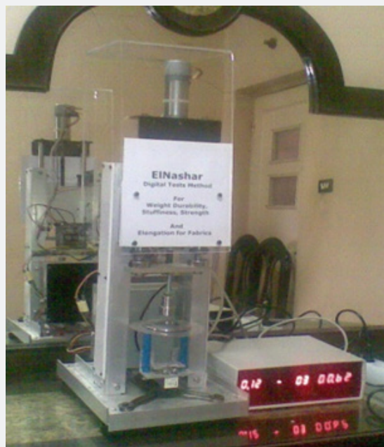
Figure 11: EInashar Digital Test method for: Weight, Durability, stuffiness, Strength and Elongation of fabrics. In EGYPT.
